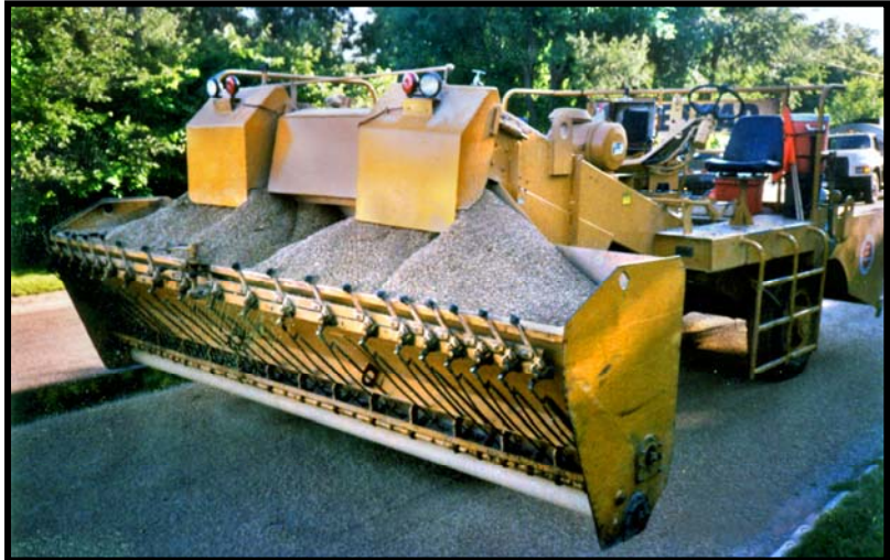
Photo 1 – Front view of the rock-chip spreading machine, showing the hoppers for the chips, the operator's seat position, and the inherent blind spot at the right front corner of the machine.
