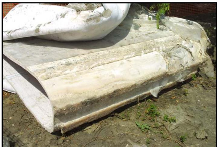
**Photo 2** – Section of uncurved fiberglass liner.
