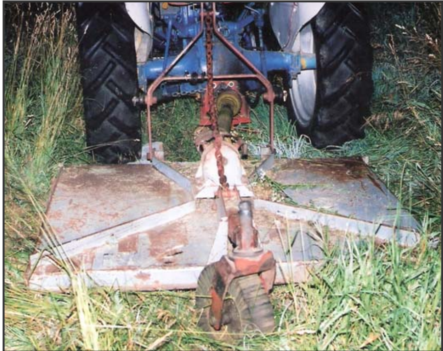
Photo 1 – PTO-powered rotary cutter attached to the tractor's three-point hitch.
