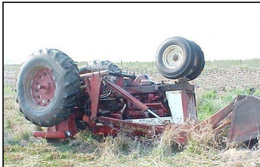
Photo 1 – Tractor without ROPS at scene of overturn. Note the rocks spilled from the loader bucket and height of the loader bucket relative to the tractor's hood.
