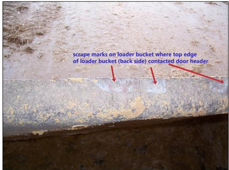
**9. Scrape marks on top edge of loader bucket.**
