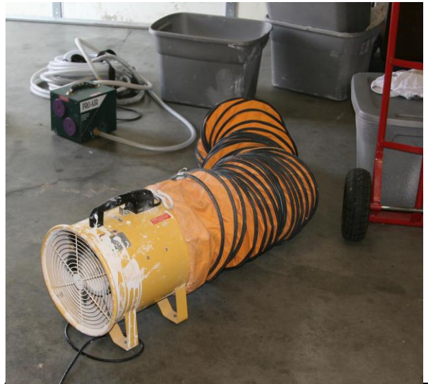
Exhibit 3: FlowPro utility blower (in foreground) was to be used to exhaust chemical vapors from the work area
