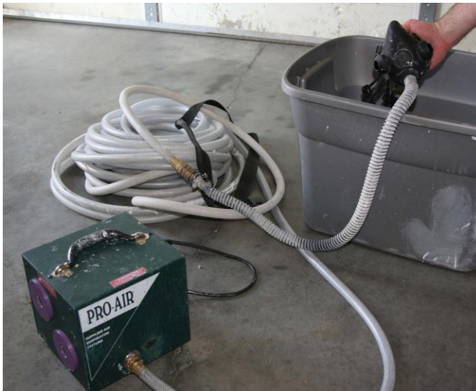
Exhibit 2: ProAir 40 Fresh Air Respirator was to be used while stripping bathtub surface
