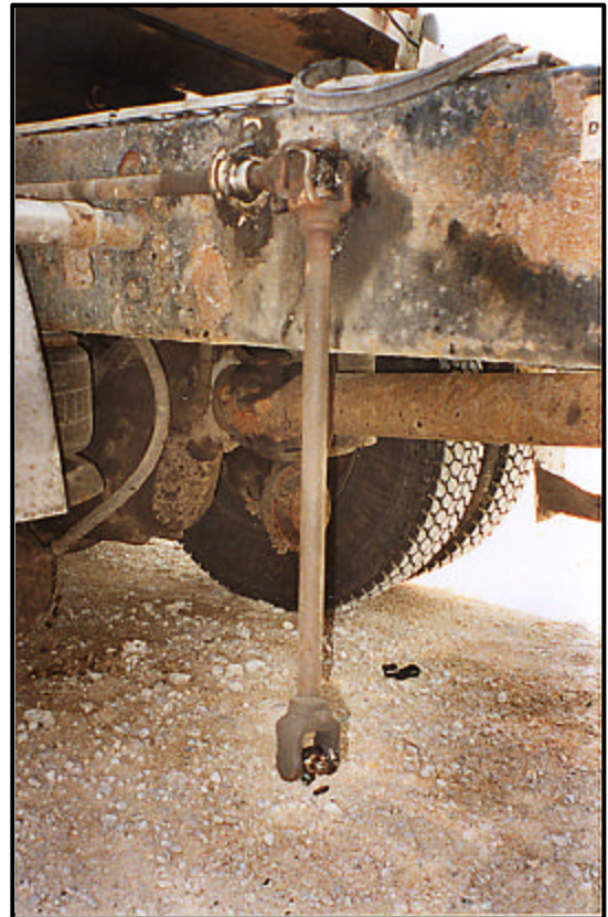
Photo 3 -- Close-up of broken PTO shaft. 1
