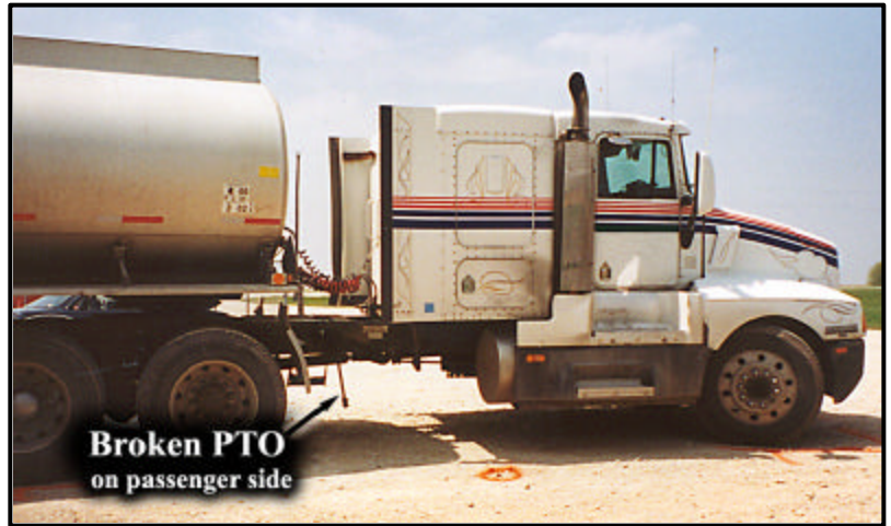
Photo 2 -- Passenger side of truck showing broken PTO shaft. 1
