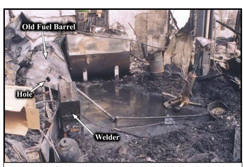
Photo 1 – View of the burned out shop area, showing the old fuel barrel and welder.
